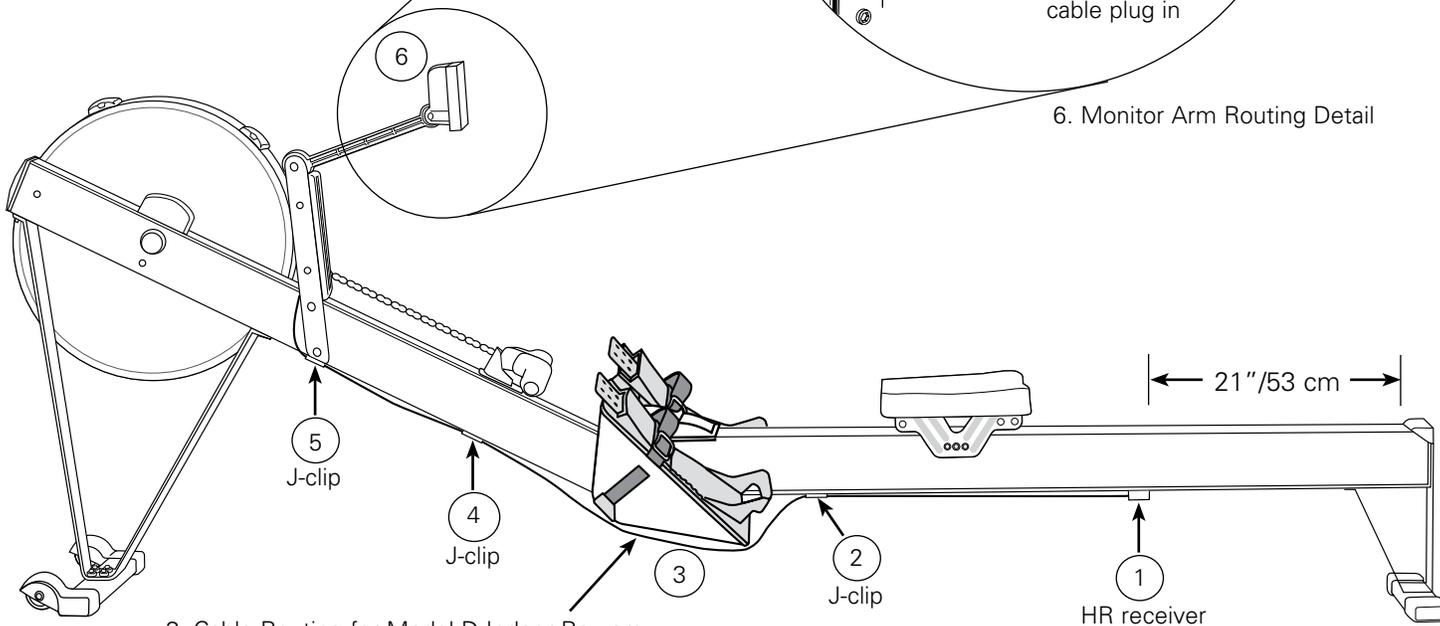
3. Cable Routing for Model D Indoor Rowers
