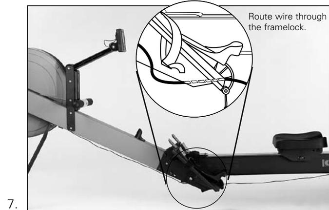
\*A. Routing for machines built before Oct. 1, 1997.
