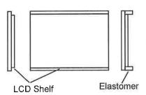
5) Place Elastomer strips on LCD shelves (see diagram at left) Clean Elastomer strips with Isopropyl Alcohol and let dry completely. Lay one Elastomer strip on either LCD shelf so that the conductive carbon contacts the LCD pads. (Do not touch the conductive portion of the Elastomer strip with bare hands). The Elastomer strips are longer than the LCD to make alignment less critical.
